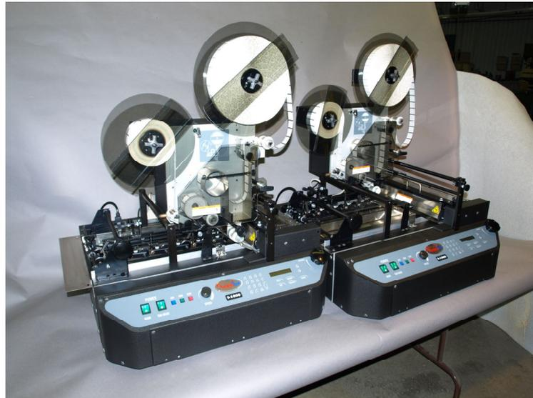
The Ameritek T1000 can also be configured as a Dual Tabber. This system can tab on the leading (toe) and trailing (heel) edges of a booklet in a single pass. The Dual Tabber can run in-line or off-line as a system, or the tabbers can be unlocked and used as standalone units.
