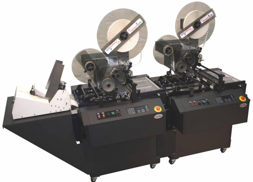
The Ameritek Tabber can also be configured as a Dual Tabber. This system can tab on the leading (toe) and trailing (heel) edges of a booklet in a single pass. The Dual Tabber can run in-line or off-line as a system, or the Tabbers can be unlocked and used as standalone units.
